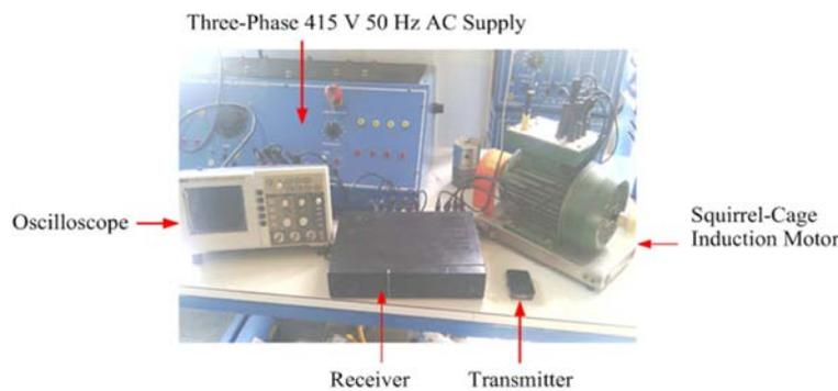
Figure 7. Setup for Testing the Transceiver System.
